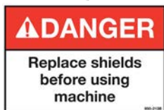
placed under belt shields
