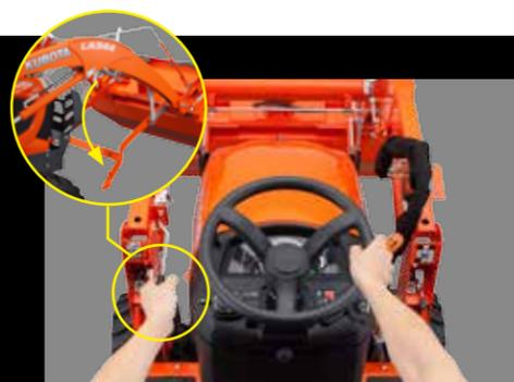
**Step 1:** Lift the loader boom and fully dump the bucket. Pull stand release lever to lower the front loader stand. Reposition the bucket so that it is in slightly dumped (20 degrees dump position) and lower the boom until the front axle is off the ground.
